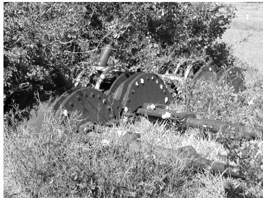
Figure 58. Silo 32B lift ring (left) and lift ring pulley mechanism (right) (ERDC-CERL).
