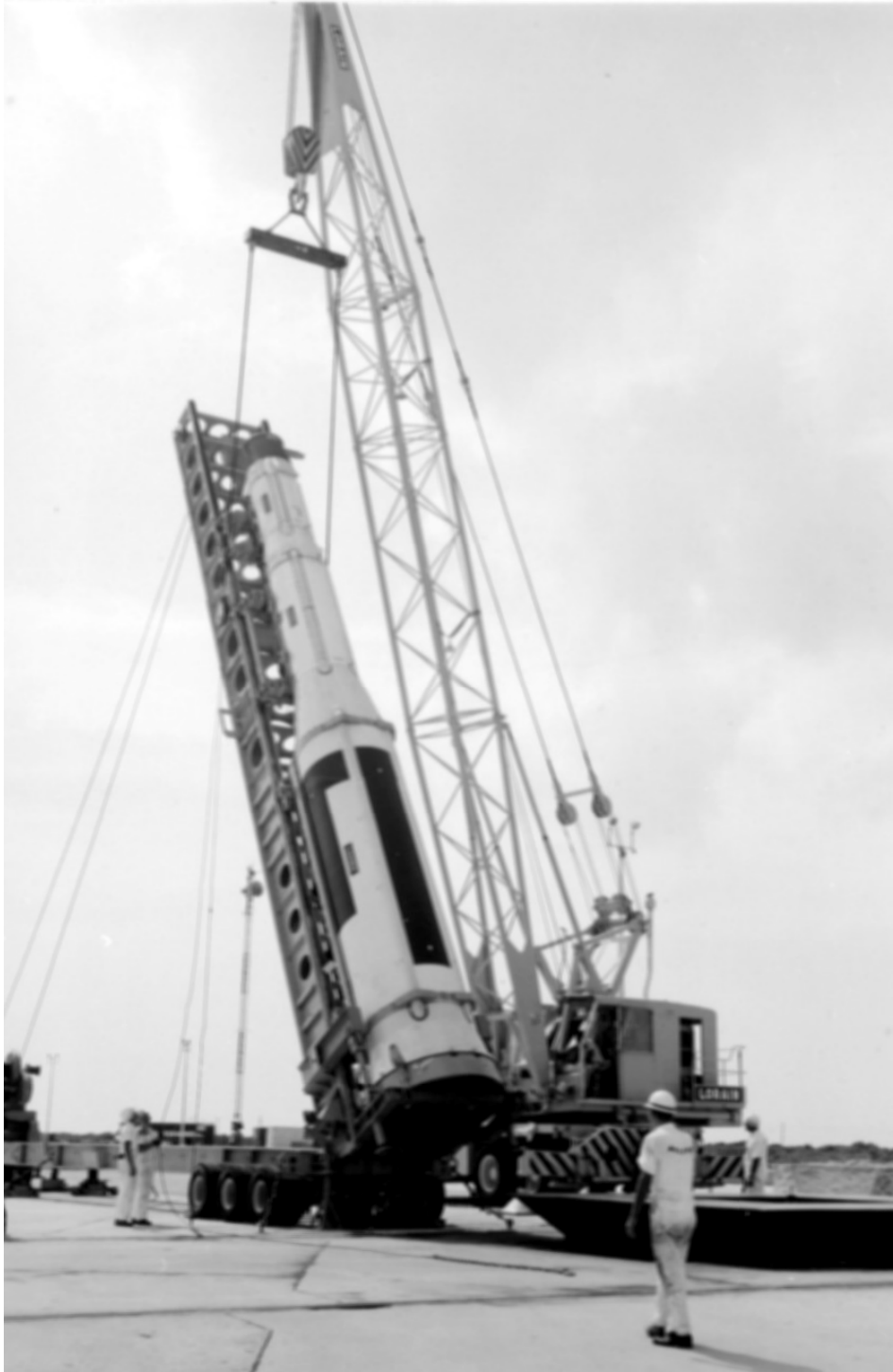
Figure 30. Minuteman I lifted by crane from transporter/erector to launcher, 12 May 1961 (NARA).
