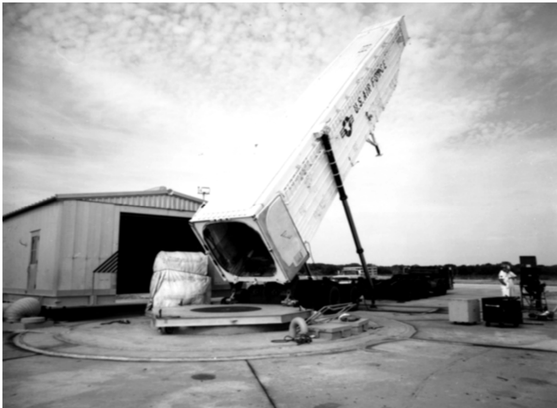
Figure 35. Transporter/erector in use for Minuteman III at silo 32B, 19 May 1970 (NARA).
