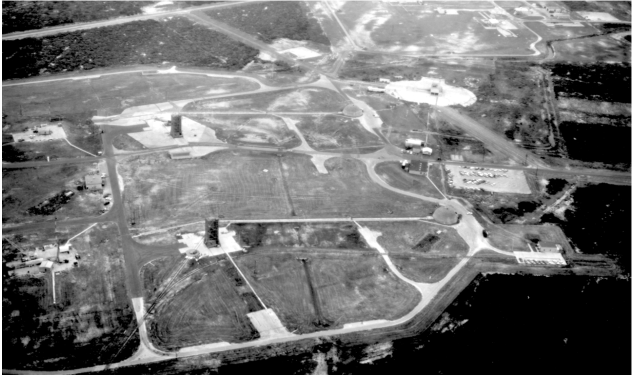
Figure 20. Aerial view of completed Complex 31/32 with silos at left, launch pads in the center, and blockhouses at right, October 1962 (NARA).
