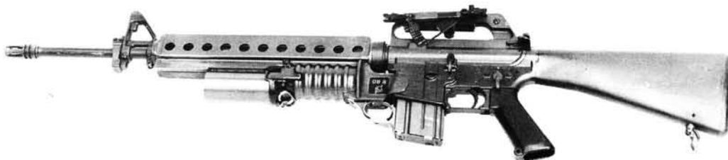
The standard M16A1 used by the US Army with a XM204 40mm Grenade Launcher (Author)
