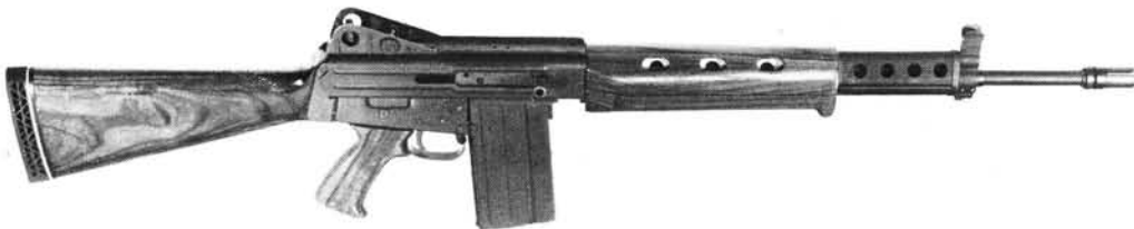
AR-16. This was a 7.62mm designed for ease and cheapness of production using the minimum of machine tools. It was not manufactured in quantity ( Armalite Inc )
