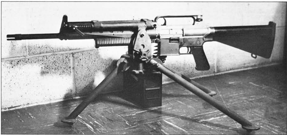
The AR-10 belt fed mounted on a tripod. The belt can just be seen feeding into the right hand side ( Armalyte Inc )
